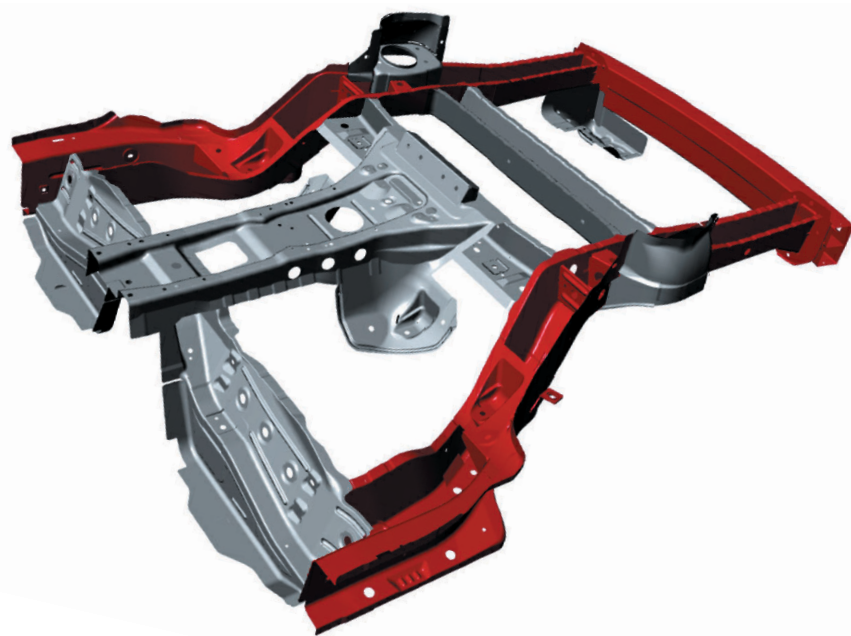
body rear structure - rear side members have a large cross-section and straight shape
