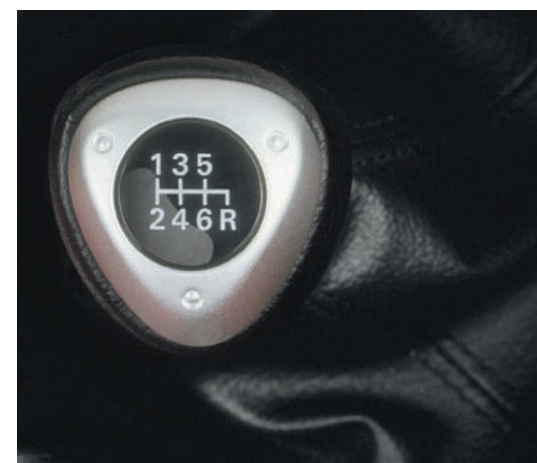
rotor shaped shift knob for 6-speed manual
