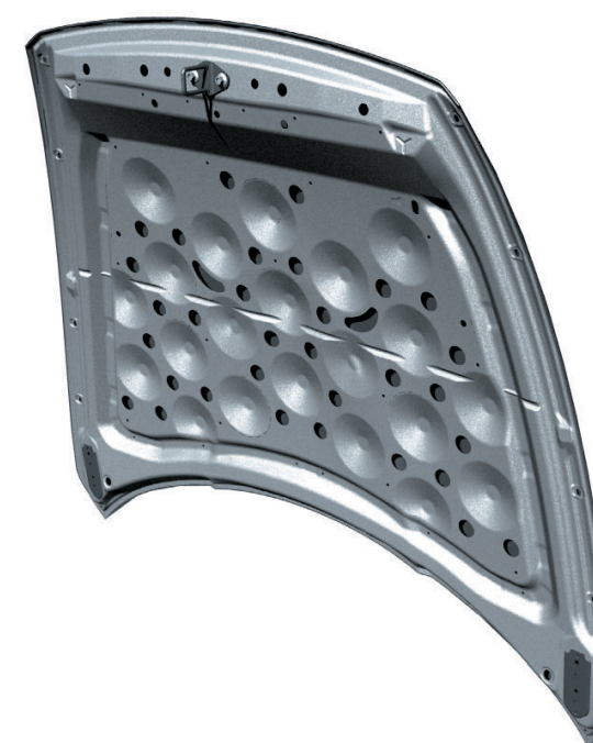
impact absorbing cone structure aluminium hood
